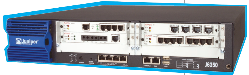
Avaya IG550 Integrated Gateway in Juniper J6350 Router.
